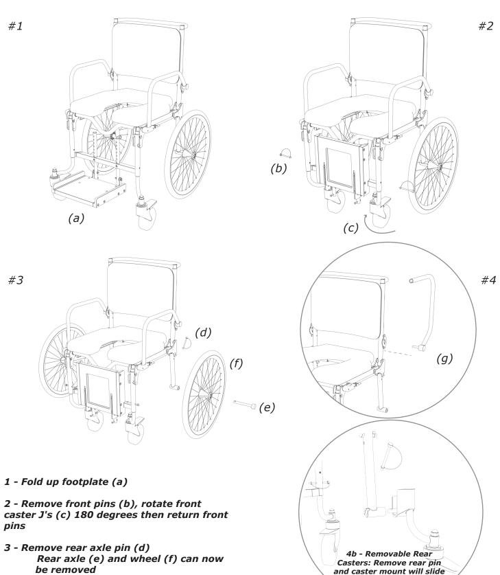
4 - Lift armrest (g) to vertical position. Armrest can now be removed out
